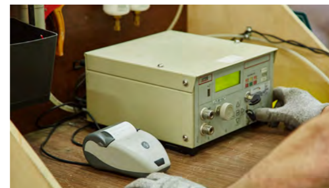
Gas system inspection by certified staff according to the German DVGW protocol.
