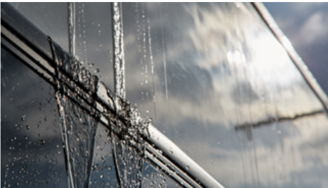
Waterproofing tests on 100% of the vehicles produced, before delivery.
